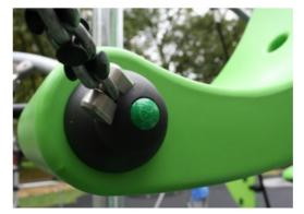
Larger activities are made of 100% recyclable PE. The play shell displayed is molded in one piece with a minimum 5mm wall thickness. PE has high impact resistance across a wide temperature span which ensures vandal resistance in all locations
