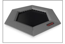
The tiles are molded in grey granulated recycled rubber (SBR/NR), and the KOMPAN logo is made of EPDM Ethylene Propylene Diene Monomer. Inside each of the rubber tiles there is a 3 mm hot dip galvanized steel plate.
