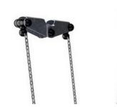
The double steel yoke suspension provides the unique parallel movement of the seat. The swing hangers are made of high quality UV stabilized nylon (PA6) housing with integrated lifetime sealed ball bearings. The height adjustable chains are fixed by a stainless steel hook with theft proof snake eye bolt in a turn able anti twist housing.
