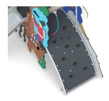
Curved climbing wall is made of Ekogrip® panel that consist of a 15mm thick PE base with 3 mm top-layer of soft rubber with a non-skid effect.
