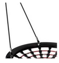
Ropes are made of UV-stabilised PA with inner steel cable reinforcement. The rope is induction treated in order to create a strong connection between steel and rope which leads to good wear resistance.
