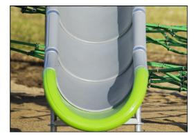
Molded PE slides made with 33% postconsumer materials in different colors in onepiece design with a wall thickness of minimum 5mm. The PE is tested for UV stability and has excellent impact strength and it is usable within a large temperature span.
