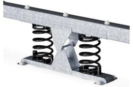
KOMPAN Springs are made of high quality spring steel according to EN10270. The springs are cleaned by phosphating before they are painted with an epoxy primer and a polyester powder coating as top finish. The springs are fixed by unique anti pinch fittings for maximum safety and long lifetime.
