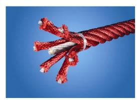
Ropes of UV-stabilized PES rope strands with inner steel cable reinforcement. The polyester yarn is made from +95% post-consumer materials and is inductively melted onto each strand. The ropes are highly wear-and vandalism-resistant and can be replaced at site if needed.
