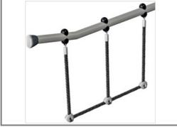
The ropes have six-stranded steel wires and a steel wire core. Each strand is tightly wrapped with PES yarn, which is melted onto each individual strand and made from +95% postconsumer materials. Climbing cable nets are completely factory assembled in a configuration that is ready for attachment to the frame on site.
