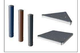
The main posts are made of high quality pregalvanized steel with powder coated top finish. Post tops are closed with caps of UV stabilized nylon (PA6). The grey colored molded decks are made of 75% post-consumer waste PP material with a non-skid pattern and texture surface. All decks are supported by unique designed low-carbon aluminum profiles with multiple attachment options.
