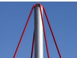
In the centre of the net is the mast which is made of high-guality seamless steel and creates an oscillating support structure which is statically favourable and equalises the oscillations in the net. The masts are hot-dip galvanised as standard, with the design option of additional powder coating.
