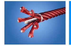
Corocord ropes with 19mm+ diameter are known as a 'Hercules' rope type which is formed from galvanised six-stranded steel wires. Each strand is tightly wrapped with PES yarn, which is melted onto each individual strand. Ropes are highly wear-and vandalism-resistant and can be easily replaced on-site if needed.
