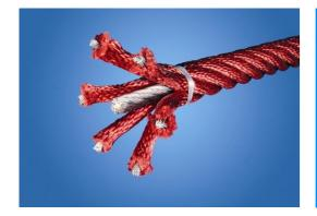
Corocord ropes with 19mm diameter or more are special 'Hercules' - type with galvanized sixstranded steel wires. Each strand is tightly wrapped with PES yarn, which is melted onto each individual strand. The ropes are highly wear-and vandalism-resistant and can be replaced at site if needed.
