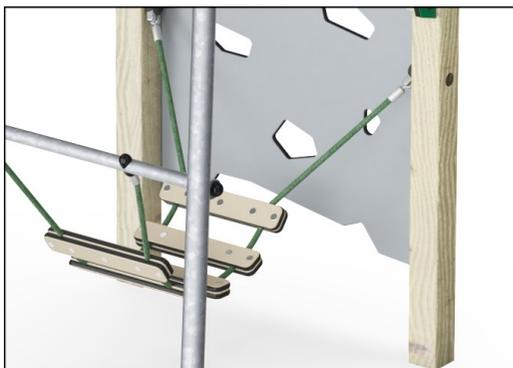
Corocord ropes of UV-stabilized PES rope strands with inner steel cable reinforcement. The polyester yarn is made from +95% post-consumer materials and is inductively melted onto each strand. PES has high strength with excellent resistance to abrasion and UV radiation. The hammock boards are made of EcoCore HDPE material made from +95% Post-consumer materials.
