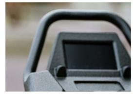
The handle bars are designed with multiple hand positions to accommodate different postures and riding styles. It is a casted aluminium part with polyurea coating for good grip and insulation.
