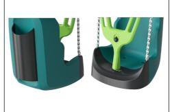
The front bumper is made with a core of strong polypropylene (PP) with a softer outer layer of thermoplastic rubber (TPE) and the rear bumper of 8mm thick EPDM membrane. The soft, shock absorbent bumpers with nonslip surface makes the swing seat extremely safe to use by caretakers.
