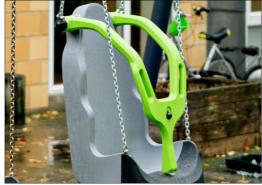
The Harness is made of moulded recyclable polyethylene (PE) made from 33% postconsumer materials. The harness utilises a stainless-steel torsion spring which makes the harness stay in position to secure easier entry and exit of users. The harness lock is designed with a one-handed operation slider made from stainless steel.
