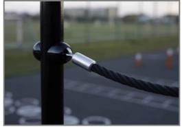
Ropes are made of UV-stabilised PES with inner steel cable reinforcement. The polyester yarn is made from +95% post-consumer materials and is inductively melted onto each strand, leading to good wear resistance.
