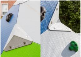
Die-casted corner brackets of high quality lead free aluminium. The corner brackets have nicely rounded edges and countersunk stainless steel screws. For sunny environments the corner brackest can be supplied with optional powder coating which reduced the heat absorption of the brackets.
