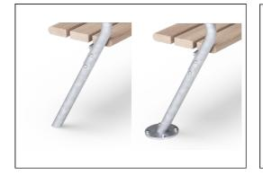
KOMPAN outdoor furniture is available for surface and in-ground installation. Surface installation by anchoring to the base layer or inground installation as either direct in ground or additional hot dip galvanized steel brackets.
