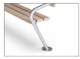
Steel internal surfaces are hot-dip galvanised, and the outside surfaces are lead and zinc free. Galvanisation has excellent corrosion resistance within outdoor environments and requires very little maintenance. Painted steel parts are hot-dip galvanised and then powder coated.
