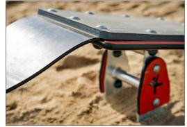
Corocord membranes consist of friction-proof rubberized material of conveyor belt quality with excellent UV resistance. Tested and compliant with REACH requirements for PAH. Embedded is a four-layered armouring made of woven polyester. The armouring and the two surface layers result in a total thickness of 8 mm.
