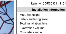
Installation Information Max. fall height 100 cm Safety surfacing area 71.0 m<sup>2</sup> Total installation time 14.3 Excavation volume 7.00 m<sup>3</sup> Concrete volume 4.90 m<sup>3</sup> Footing depth (standard) 110 cm Shipment weight 491 kg Anchoring options In-ground
