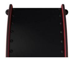
Membranes consist of friction-proof rubberized material of conveyor belt quality with excellent UV resistance. Embedded is a four-layered armouring made of woven polyester. The armouring and the two surface layers result in a total thickness of 9 mm.
