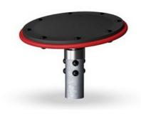
The upper plate is manufactured from Ekogrip® panel that consists of a 15mm thick PE base with 3 mm top-layer of soft rubber with a non-skid effect.
