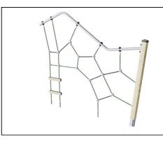
Corocord ropes of UV-stabilized PES rope strands with inner steel cable reinforcement. The polyester yarn is made from +95% postconsumer materials and is inductively melted onto each strand. PES has high strength with excellent resistance to abrasion and UV radiation. The rope loops are assembled by aluminum connectors.
