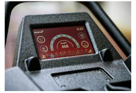
The durable 7" LCD, touchscreen with IK8 protection glass gives instant feedback on speed, distance, time, burned calories etc. The resistance of the crosstrainer can be adjusted on the screen.
