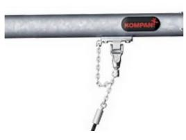
KOMPAN heavy duty designed swing hangers of stainless steel with anti-twist function. The hangers are attached to the cross beam on a welded bracket with two bolts, The bearings are embedded with silicone lubricant and needs no further lubrication.
