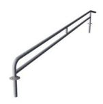
The railing height is 930mm, and the distance between the railing is 900mm The material used for the railing is hot-dip galvanised steel ø38 mm, a great diameter for a good grip and wrist support.
