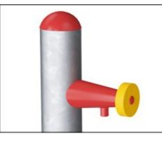
The integrated water tap open for water when pushed and stops when letting go. The water is supplied trough a pipe located inside the post with hose or pipe connection at the bottom of the post. The supply can either be a loose hose or a permanent in-ground pluming.
