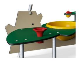
Play activities like the Funnel are made of injection moulded high quality nylon (PA6). PA6 has good wearing and impact strength and is UV stabilised.
