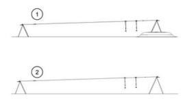
KOMPAN cableways are available for flat or natural sloped surroundings and for surface or in-ground installation. Further the cableways can be supplied with one or two cables for children to ride together in friendly competition.
