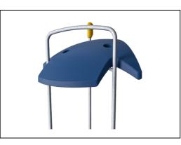
The ELEMENTS roofs are made of recyclable PE with a minimum wall thickness of 5 mm to ensure high durability in all climates around the world. The steel pipes are hot-dip galvanised inside and outside for maximum durability.
