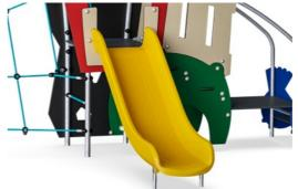
Molded PE slides made with 33% postconsumer materials in different colors in onepiece design with a wall thickness of minimum 5mm. The PE is tested for UV stability and has excellent impact strength and it is usable within a large temperature span.
