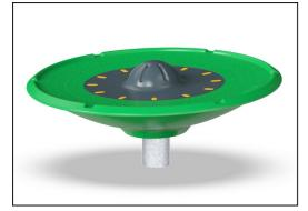
The outer ring of the Spinner Disc base is made of recyclable LDPE. The ring is molded in one piece with integrated metal thread bushings and water drain holes to ensure high durability in all climates around the world.
