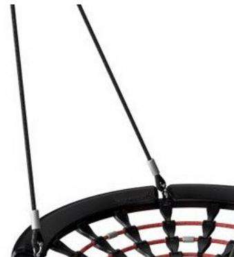
KOMPAN heavy duty designed swing hangers of stainless steel with anti-twist function. The hangers are attached to the cross beam on a welded bracket with two bolts, The bearings are embedded with silicone lubricant and needs no further lubrication.
