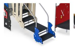
All floors are made of High-Pressure Laminate HPL with a thickness 17.8mm and non skid surface texture according to EN 438-6. KOMPAN HPL has high wearing strength to ensure long lifetime in all climates.
