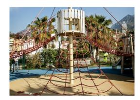
Corocord 16mm ropes of UV-stabilized PES rope strands with inner steel cable reinforcement. The polyester yarn is made from +95% post-consumer materials and is inductively melted onto each strand. The ropes are highly wear-and vandalism-resistant and can be replaced at site if needed.
