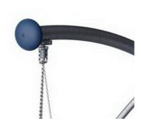
Unique designed 360-degree rotating swing hanger made of stainless steel. The moving parts of the swing hanger is lifetime sealed and lubricated. The hanger system is equipped with a safety chain to prevent the swing hanger to fall down if damaged.
