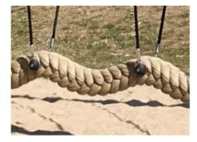
The rope of the pendulum swing is made of polypropylene (PP) rope in Coconut style with a square shape of 14x14cm. The ends of the Coconut rope are closed by a steel clamps and sealed by a glued-on shrinkable tubing. The last 10cm of the rope ends are cut open to make a tassel with bumper function to fulfill global safety requirements.
