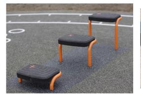
The support frame is ø48.3 x 4mm, carbon steel, with a hot-dip galvanized surface according to ISO1461, and a powder coating corrosion class C3 according to ISO12944-2. Lead content for surfaces are below 90ppm.
