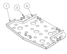
A 5 mm hot-dip galvanized carbon steel plate must is molded inside the SBR to offer optimal stability and optimize the mounting of the step to the frame.
