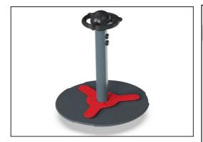
A heavy-duty engineered bearing system with two single row deep groove high-quality ball bearings with rubber seals. The fully closed bearing construction is lifetime lubricated and located above ground.
