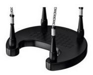
KOMPAN designed curved toddler seat is made with an insert of 21.25 mm thick plywood from alder and pine wood. The outside layer is molded in UV stabilized PUR which retains its properties in the temperature range of -30°C to 60°C.
