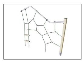
The rope nets are made of single braided 16 mm PES ropes. PES has high strength with excellent resistance to abrasion and UV radiation. The rope loops are assembled by aluminum connectors.
