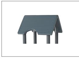
Roof is made from rotomolded PE. PE has high impact resistance across a wide temperature span that ensures durability. The steel surfaces are hot-dip galvanized inside and outside with lead-free zinc. The galvanization has excellent corrosion resistance in outside environments and requires minimal maintenance.
