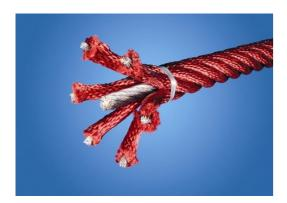
Saturn ropes are manufactured from a with a six-stranded steel wire core that is tightly wrapped with PES yarn which is melted onto each strand. A second surface coat of harder PES is also applied, to ensure the rope is highly durable and vandalism-resistant.
