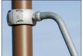
Colored steel components have a base of hot dip galvanization and a powder coated top finish. This provides an ultimate corrosion resistance in all climates around the world. Other steel surfaces are hot dip galvanized inside and outside with lead free zinc.
