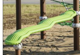
Rocking tube is made of medium density PE with excellent impact strength and usable within a large temperature span. Hollow plastic components are made of 100% recyclable PE made from 33% post-consumer materials. Molded in one piece with minimum 5mm wall thickness. The longitudinal grooves provides a slip resistant surface for safe play.
