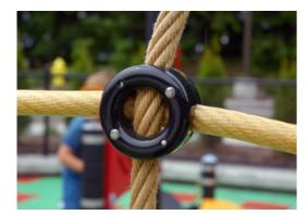
Climbing nets are made of UV-stabilised PA rope with inner steel cable reinforcement. The rope is induction treated to obtain maximum fixation between steel and rope, which provides excellent wear and tear resistance. All rope connectors are made of 100% recyclable PA material.
