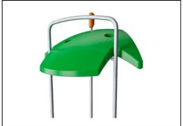
The ELEMENTS roofs are made of recyclable PE made from 33% post consumer recycled materials with a minimum wall thickness of 5 mm to ensure high durability in all climates around the world. The steel pipes are hot dip galvanised inside and outside for maximum durability.
