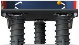
KOMPAN's springs are manufactured from highquality spring steel. The springs are cleaned by phosphating before being painted with epoxy primer and polyester powder coating. The springs are fixed by unique anti-pinch fittings for maximum safety and longevity.
