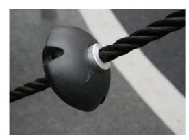
GALAXY ropes has six-stranded steel wires and a steel wire core. Each strand is tightly wrapped with PES yarn, which is melted onto each individual strand. The PES yarn is made of +95% Post-consumer materials to obtain excellent wear and tear resistance.
