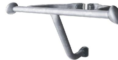
The support handle is 530mm wide. The handle is 1050mm above ground level, and 1140mm above the jumper membrane. The handle is made from an Ø32mm HDG bar.
