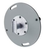
The bearing house is made from hot dip galvanised steel. The bearing shaft is made from stainless steel AlSI304. The bearing itself is made from Polyoxymethylene (POM), an engineering thermoplastic with a high stiffness, low friction, and excellent dimensional stability.
